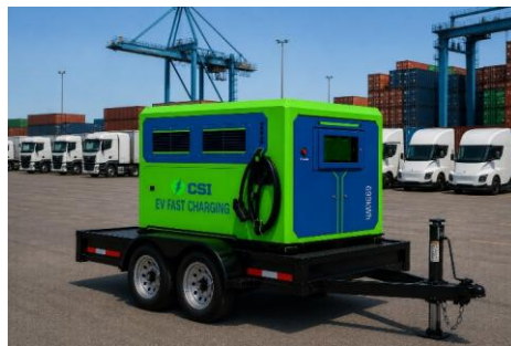
CSI's 699 kWh Mobile BESS with Integrated MCS
